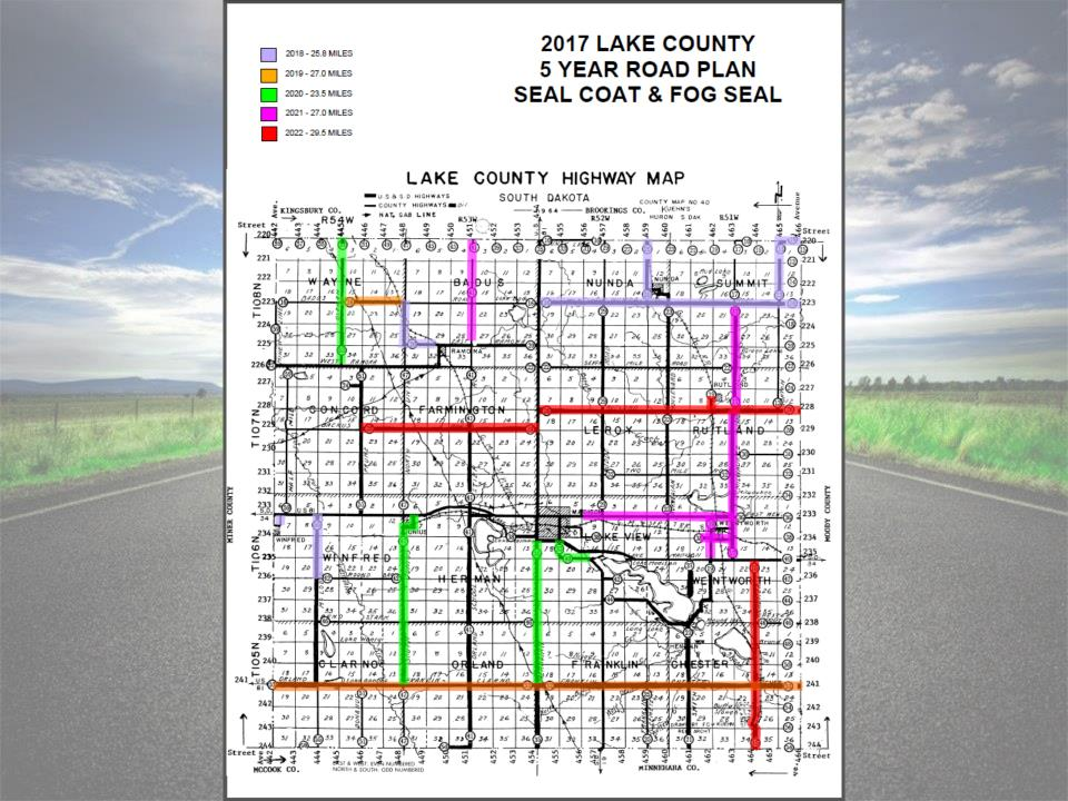
FIVE-YEAR PROGRAMMED PROJECT LISTING(Sealcoating Rate .35 sq/yd CRS-2P #8 Red Chips)INCLUED FOG SEAL
